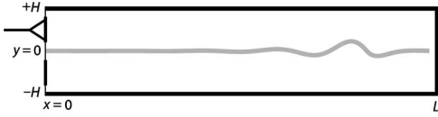
FIG. 3. Spacetime slice through a symmetric, two-dimensional box model of height H . The x axis extends longitudinally from the base ( x=0 ), and the y axis is oriented perpendicular to the basilar membrane, which spans the entire width, b , of the cochlea. The snapshot shown here has caught the BM participating in a traveling wave, whose vertical displacements have been hugely exaggerated for the purposes of illustration. The inversion procedure described in the text finds the wave's propagation and gain functions by analyzing measurements of the spatial displacement pattern.
